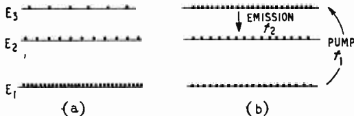
Fig. 6 Three Zeeman levels are shown here, with relative numbers of electrons in them indicated, (a) without excitation, (b) with excitation.
